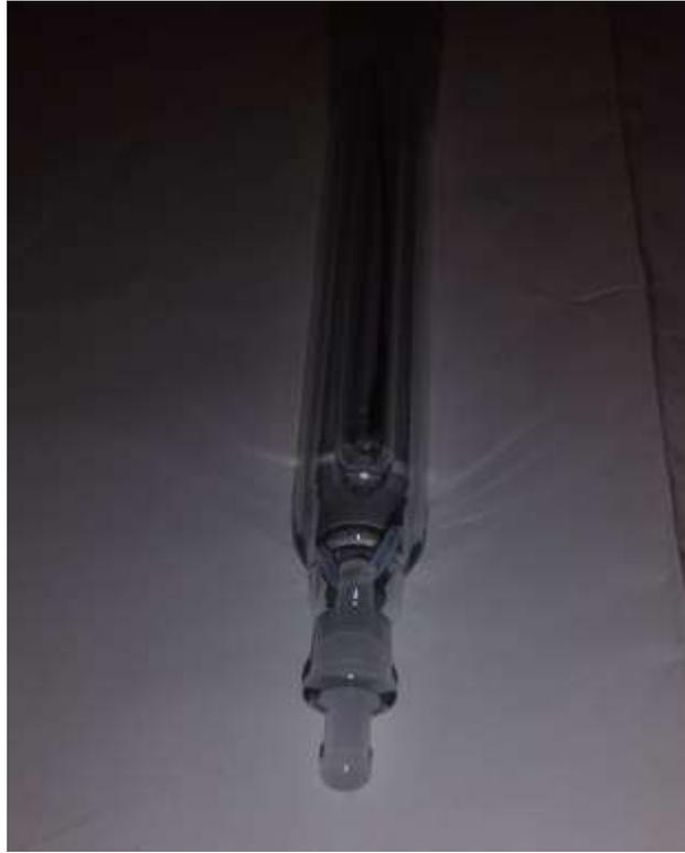
**Figura 30. Punta Semipermeable Ag/AgCl**
